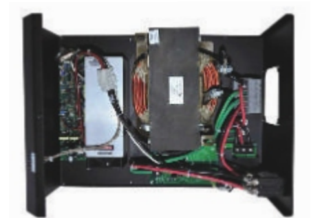
Top view showing the transformer, control board and surge protection/filter board components
