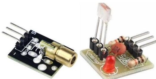
Figura 3.5 Módulo sensor laser KY-008
