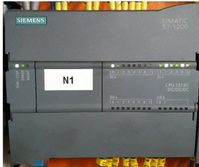
**Figura 1.5: PLC Siemens S7-1200, CPU 1214C, DC/DC/DC**
