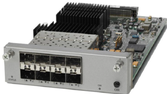
Figure 3. 8 x 10 Gigabit Ethernet Port Uplink Module
