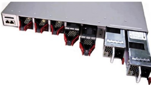
Figure 6. Redundant Fan and Power Supply
