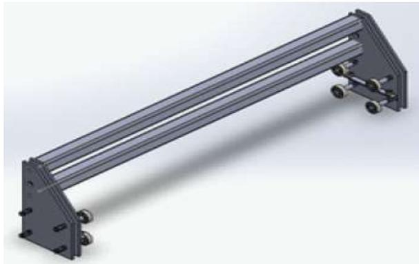
**Figura 64.** Eje lineal “X”.
